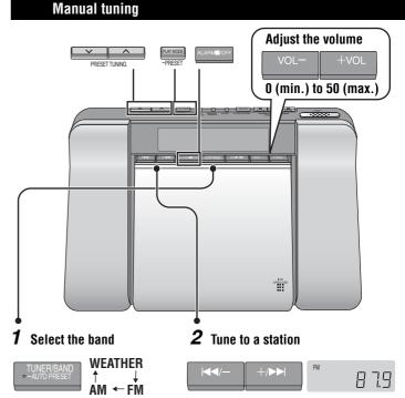
In step 2, press and hold to start automatic tuning. Tuning stops when a station is found.
