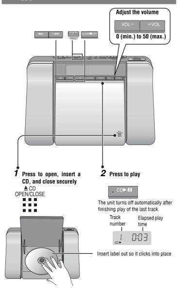
To prevent damage to the CD, stop the disc before opening the CD lid.
